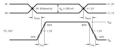
Figure 6. Receiver Propagation Delay and Transition Time Waveforms
