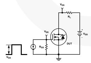
Figure 19. Switching Time Test Circuit
