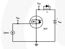
Figure 17. Gate Charge Test Circuit
