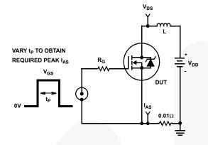
Figure 15. Unclamped Energy Test Circuit
