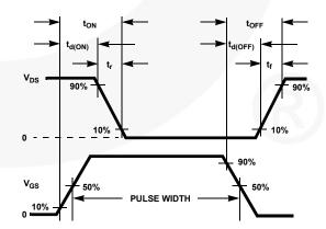
Figure 20. Switching Time Waveforms
