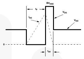
Figure 16. Unclamped Energy Waveforms
