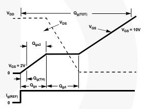
Figure 18. Gate Charge Waveforms
