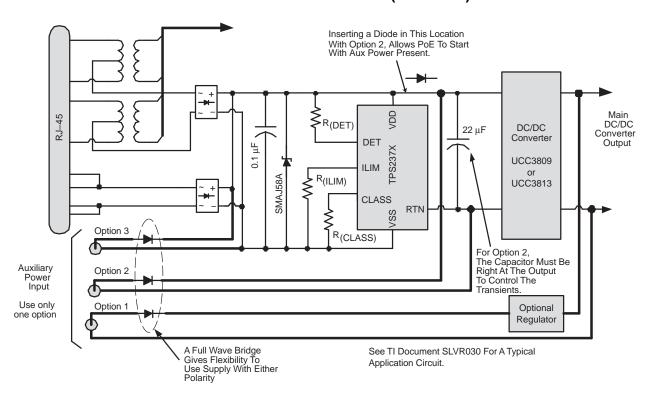
Figure 14. Auxiliary Power ORing
