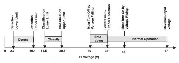
Figure 12. IEEE 802.3 PD Voltage Limits
