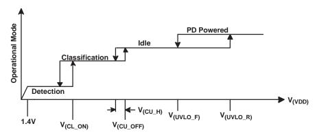
Figure 13. Threshold Voltages
