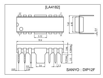
Note) In general applications, heat generated in this package can be radiated through the Cu-foiled area of the printed circuit board, but since power dissipation Pd may be increased depending on the supply voltage and load conditions, it is recommended to use a fin additionally.
