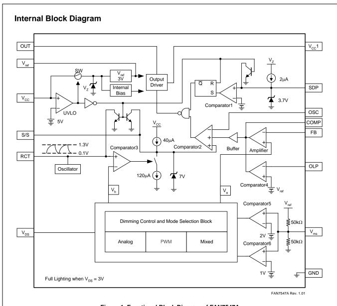
Figure 1. Functional Block Diagram of FAN7547A
