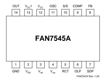
Figure 2. Pin Configuration (Top View)
