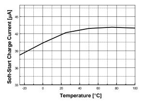
Figure 7. Soft-Start Charge Current vs. Temperature
