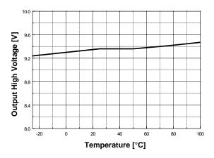
Figure 11. Output High Voltage vs. Temperature
