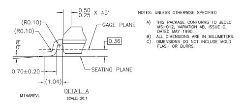
Figure 14. 14-Lead Small Outline Package (SOP)
