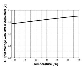
Figure 13. Output Voltage with UVLO Activated vs. Temperature
