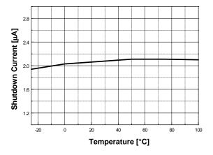
Figure 9. Protection Current vs. Temperature
