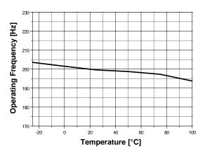
Figure 8. Operating Frequency vs. Temperature
