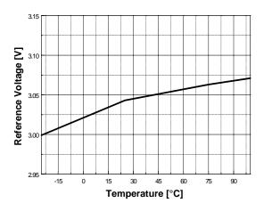
Figure 6. Reference Voltage vs. Temperature
