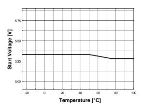
Figure 4. Start Voltage vs. Temperature
