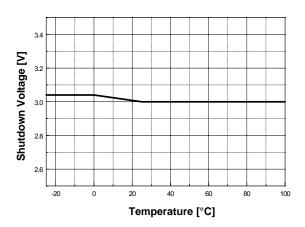
Figure 10. Protection Voltage vs. Temperature
