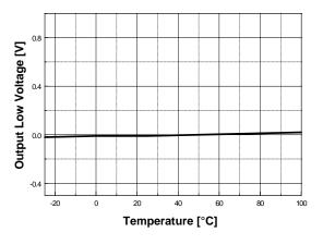
Figure 12. Output Low Voltage vs. Temperature
