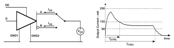
Figure 16. Driver Short-Circuit Test Circuit and Waveforms (Short Circuit applied at Time t=0)
