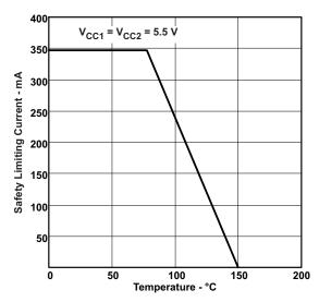
Figure 29. Thermal Derating Curve per VDE
