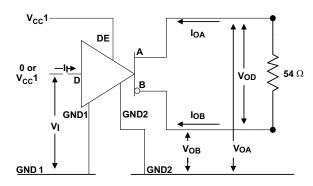
Figure 10. V<sub>OD</sub> Test Circuit
