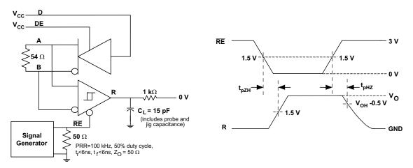
Figure 24. Receiver Enable Test Circuit and Waveforms, Data Output High
