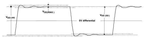
Figure 14. V<sub>OD(RING)</sub> Waveform and Definitions
