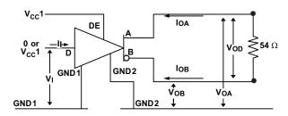
Figure 15. Input Voltage Hysteresis Test Circuit
