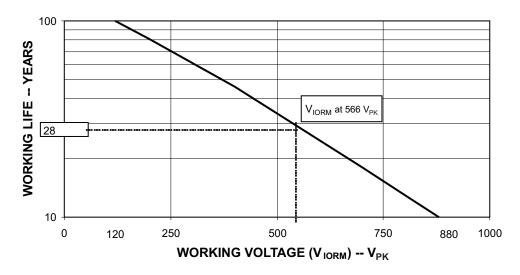
Figure 35. Time-Dependent Dielectric Breakdown Test Results
