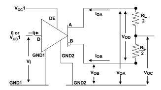
Figure 12. Driver  $V_{\text{OD}}$  and  $V_{\text{OC}}$  Without Common-Mode Loading Test Circuit
