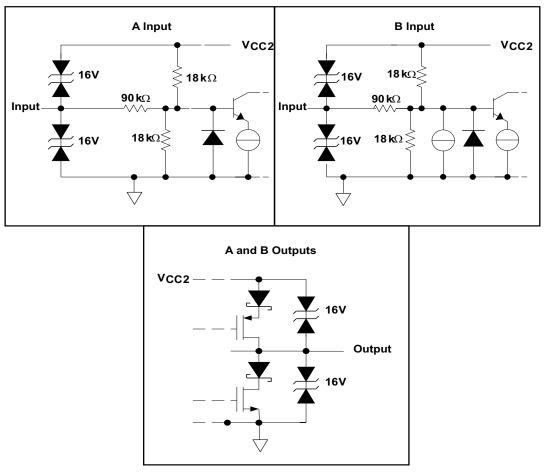
Figure 31. Equivalent Circuit Schematics
