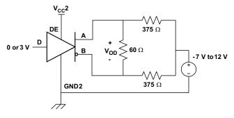
Figure 11. Driver V<sub>OD</sub> with Common-mode Loading Test Circuit
