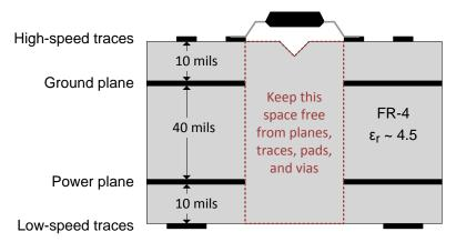
Figure 36. Recommended Layer Stack
