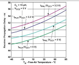
Figure 8. Receiver Propagation Delay vs Free-Air Temperature
