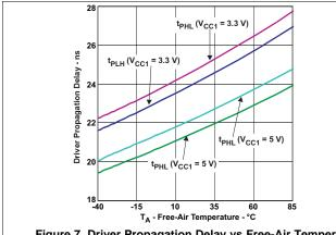
Figure 7. Driver Propagation Delay vs Free-Air Temperature
