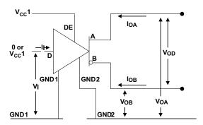
Figure 9. Open Circuit Voltage Test Circuit
