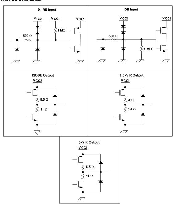
Figure 30. Equivalent Circuit Schematics
