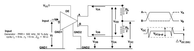
Figure 13. Steady-State Output Voltage Test Circuit and Voltage Waveforms
