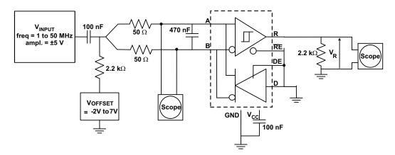
Figure 26. Common-Mode Rejection Test Circuit
