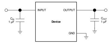
Figure 8-1. Typical Application Circuit
