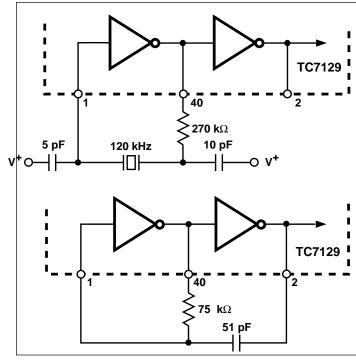
Figure 8. Oscillator Circuits
