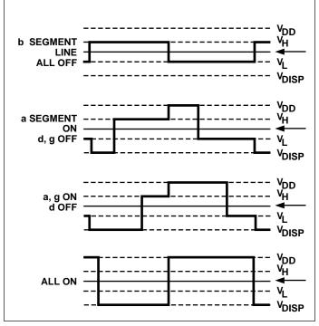
Figure 19. Typical Display Output Waveforms
