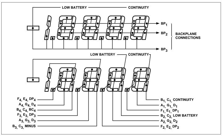
Figure 17. Display Segment Assignments
