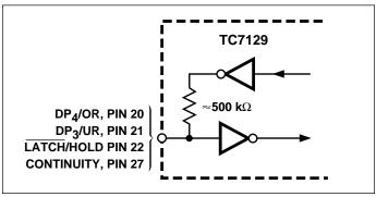
Figure 15. Input/Output Pin Schematic
