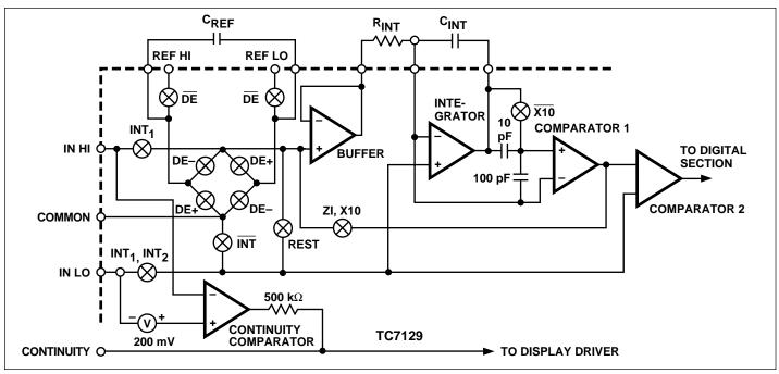
Figure 13. Integrator Block Diagram
