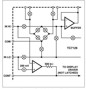
Figure 14. Continuity Indicator Circuit
