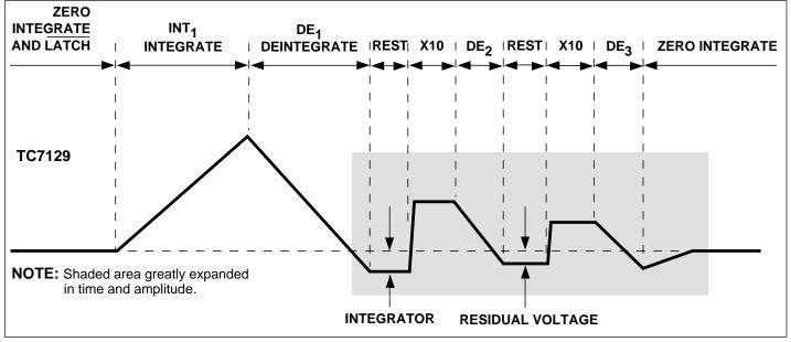
Figure 11. Integrator Waveform
