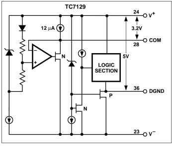
Figure 16. Digital Ground (DGND) and Common Outputs
