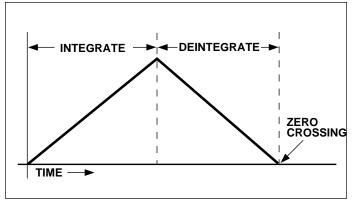
Figure 9. Dual-Slope Conversion
