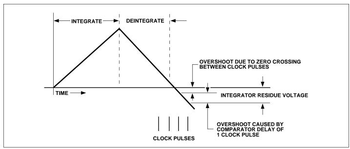
Figure 10. Accuracy Errors in Dual-Slope Conversion
