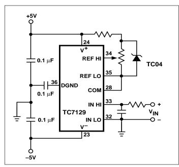
Figure 2. Powering the TC7129 From a  $\pm$ 5V Power Supply
