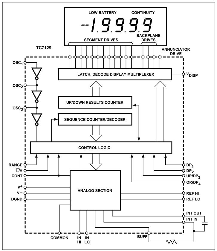
Figure 12. Functional Block Diagram
