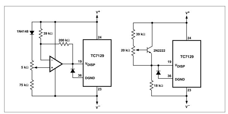
Figure 7. Temperature Compensating Circuits
