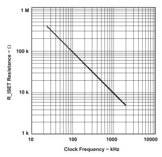
Figure 33. ISET Resistance vs Clock Frequency
