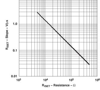
Figure 36. Slope vs RISET Resistance
