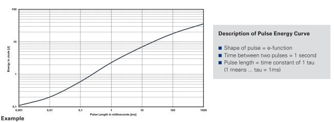
At 1 ms tau the LXP-18 with e.g. 1  $\Omega$  to 10  $\Omega$  can withstand an energy level of about 2.3 J, when the pulse pause time is  $\geq$  1s
