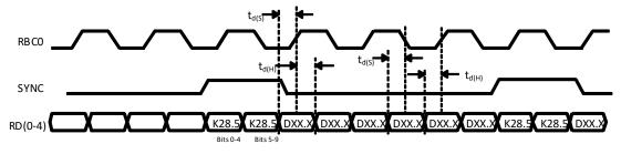
Figure 7. Synchronous Timing Characteristics Waveform (DDR mode)
