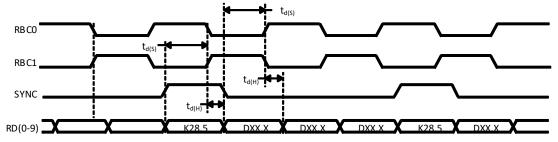
Figure 5. Synchronous Timing Characteristics Waveform (TBI half-rate mode)
