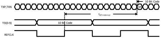
Figure 4. Transmit Latency in Full-rate Mode
