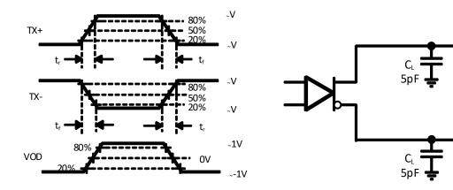
Figure 1. Definitions of Output Differential Signal and Common-mode Voltage
