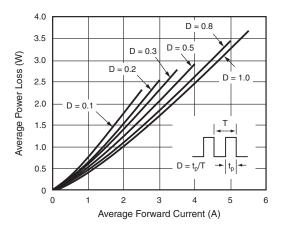
Fig. 3 - Forward Power Loss Characteristics Per Diode
