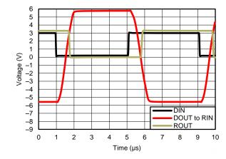
Figure 8. 250 kbit/s Driver to Receiver Loopback Timing Waveform,  $V_{CC}\text{=}$  3.3 V
