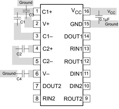
Figure 9. Layout Diagram
