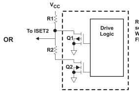
R1/R2 Divider set to 0.9 V Which is the Float Voltage
