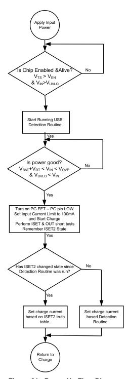
Figure 21. Power Up Flow Diagram
