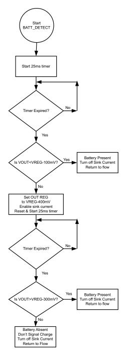
Figure 24. Battery Detect Flow Diagram
