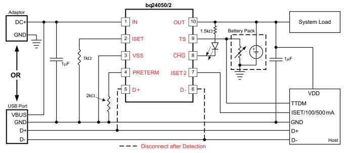
$I_{OUT\_FAST\_CHG} = 540 \text{ mA}$ ;  $I_{OUT\_PRE\_CHG} = 108 \text{ mA}$ ;  $I_{OUT\_TERM} = 54 \text{ mA}$
