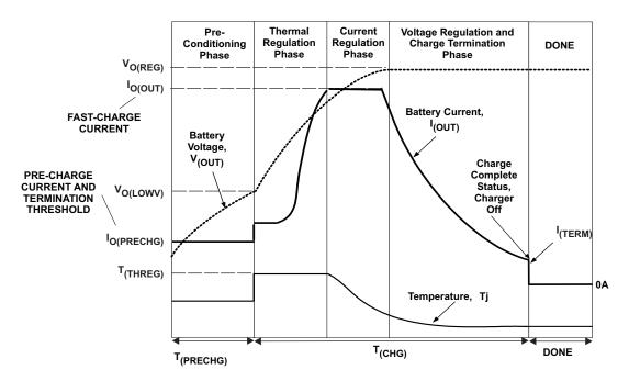
Figure 19. Charging Profile With Thermal Regulation
