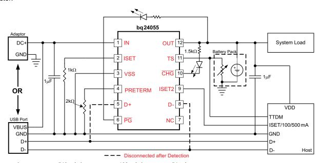
$I_{OUT\_FAST\_CHG}$  = 540 mA;  $I_{OUT\_PRE\_CHG}$  = 108 mA;  $I_{OUT\_TERM}$  = 54 mA
