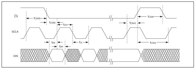
Figure 5. Detailed Serial Interface Timing Diagram
