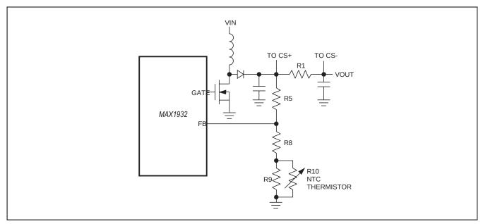
Figure 8. Adding an NTC Thermistor for Hardware Temperature Compensation; Output Voltage Increases with Temperature Rise
