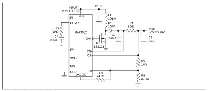
Figure 2. Typical Operating Circuit
