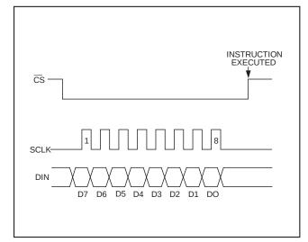
Figure 4. Serial Interface Timing Diagram
