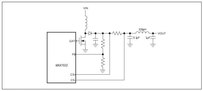
Figure 7. Adding a Post LC Filter
