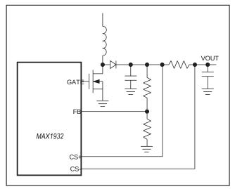
Figure 3. Taking Feedback Ahead of Output Filter
