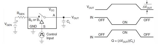
Figure 9. Charge Injection
