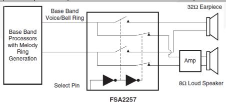
Figure 1. Block Diagram
