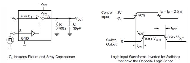
Figure 6. Turn On / Off Timing
