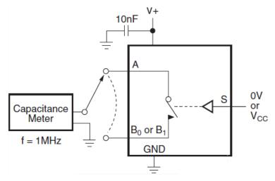
Figure 10. On / Off Capacitance Measurement Setup
