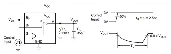
C<sub>L</sub> Includes Fixture and Stray Capacitance
