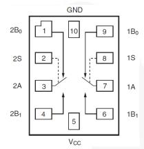
Figure 4. Pin Assignments for MSOP (Top View)
