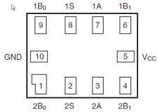
Figure 2. Pin Assignments for TSSOP (Top View)
