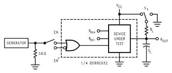
$\ensuremath{C_L}$  includes load and test jig capacitance.
