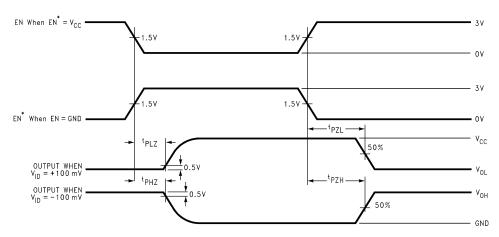
Figure 5. Receiver TRI-STATE Delay Waveforms
