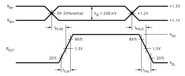
Figure 3. Receiver Propagation Delay and Transition Time Waveforms
