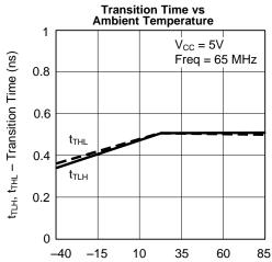
$T_A$  – Ambient Temperature ( $^{\circ}$ C) Figure 18.
