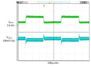
Figure 12. Load Transient, Vout=3.3V, Iout=0.75A-2.25A
