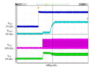
Figure 7. Startup Waveforms
