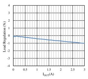
Figure 6. Load Regulation vs. Load Current
