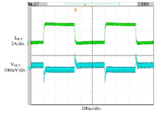
Figure 11. Load Transient, Vout=3.3V, Iout=0.1A-3A
