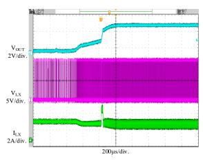
Figure 10. Short Circuit Recovery
