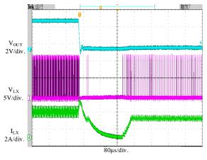
Figure 9. Short Circuit Protection
