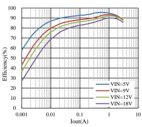
Figure 3. Efficiency vs. Load Current,  $V_{OUT} = 3.3V$
