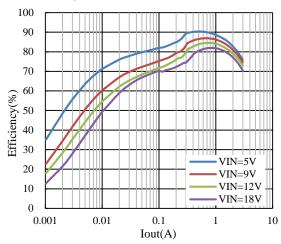
Figure 1. Efficiency vs. Load Current,  $V_{\rm OUT} = 1.2 V \label{eq:Vout}$
