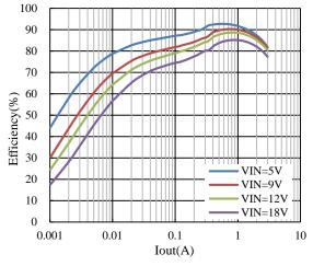
Figure 2. Efficiency vs. Load Current,  $V_{\rm OUT} = 1.8 V \label{eq:Vout}$
