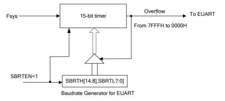
From the figure, the baud rate generator overflow rate:  $SBRToverflow rate = \frac{Fsys}{32768 - SBRT1}$ , SBRT1 = [SBRTH1, SBRTL1].
