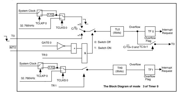
**Note:** While Timer1 is used as baud rate generator, reading or writing TH1/TL1 will affect the accuracy of baud rate, thus might make cause communication error.
