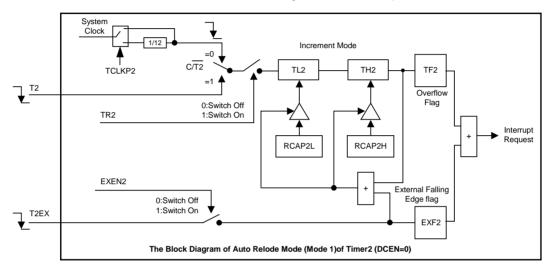
Setting the DCEN bit enables Timer2 to count up or down. When DCEN = 1, the T2EX pin controls the direction of the count, and EXEN2's control is invalid.
