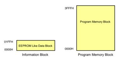
The SH79F1612B embeds 16K flash program memory for program code. The flash program memory provides electrical erasure and programming and supports In-Circuit Programming (ICP) mode and Self-Sector Programming (SSP) mode. 1024 bytes per sector.
