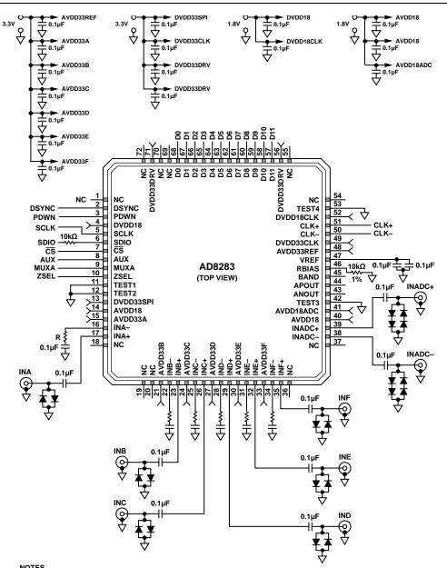
NOTES 1. RESISTOR R (INX- INPUTS) SHOULD MATCH THE OUTPUT IMPEDANCE OF THE INPUT DRIVER. 2. ALL CAPACITORS FOR SUPPLIES AND REFERENCES SHOULD BE PLACED CLOSE TO THE PART.
