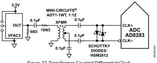
Figure 27. Transformer-Coupled Differential Clock
