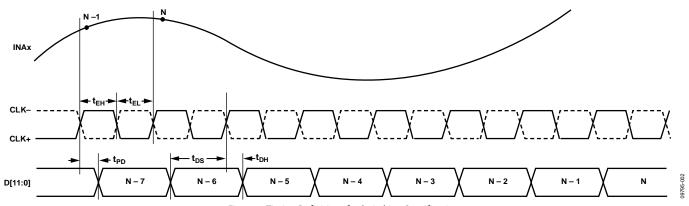
Figure 2. Timing Definitions for Switching Specifications
