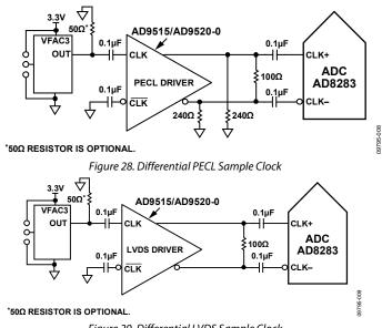
Figure 29. Differential LVDS Sample Clock
