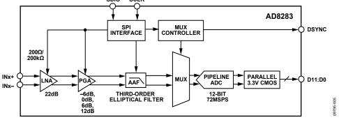
Figure 25. Simplified Block Diagram of a Single Channel
