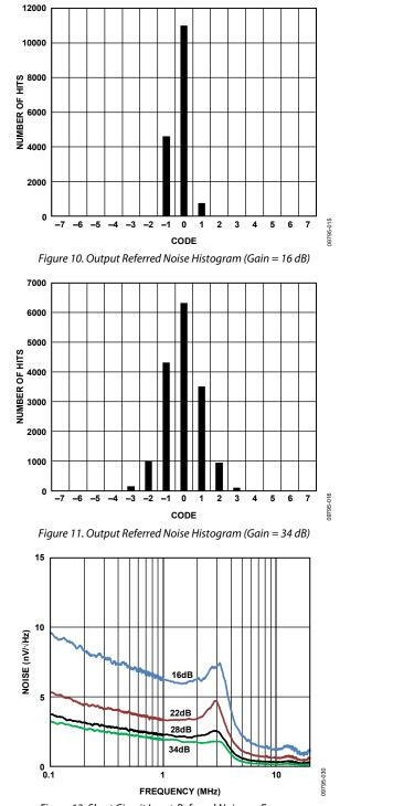
Figure 12. Short Circuit Input-Referred Noise vs. Frequency
