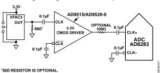
Figure 31. Single-Ended 3.3 V CMOS Sample Clock
