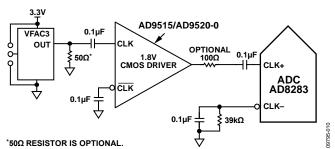
Figure 30. Single-Ended 1.8 V CMOS Sample Clock
