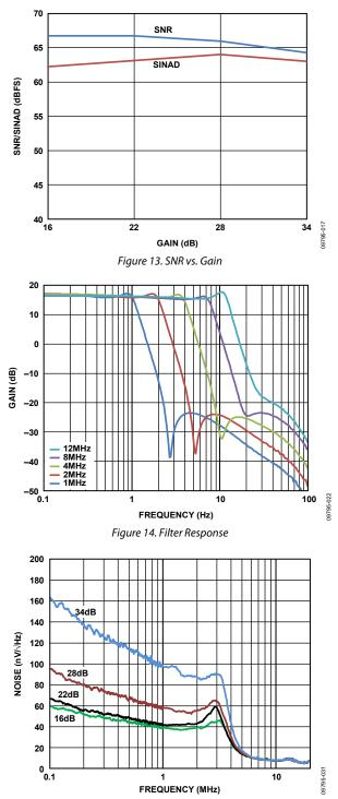
Figure 15. Short-Circuit Output-Referred Noise vs. Frequency
