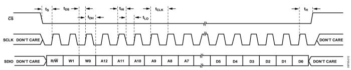
Figure 32. Serial Timing Details
