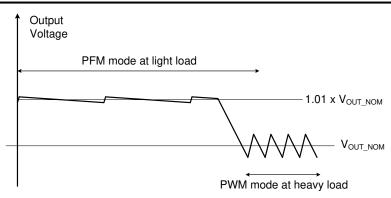
Figure 8-1. Output Voltage in PWM Mode and PFM Mode
