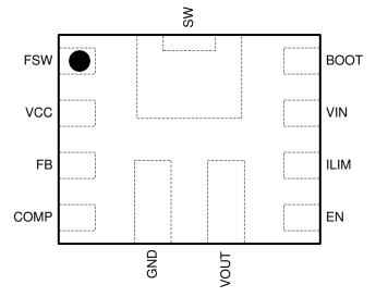
Figure 6-1. 11-Pin VQFN With Thermal Pad RNR Package (Top View)
