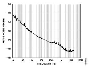
Figure 19. Additive (Residual) Phase Noise, CLK-to-LVDS at 245.76 MHz, Divide-by-1
