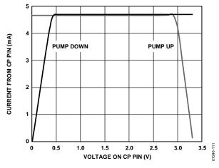
Figure 8. Charge Pump Characteristics at VCP = 3.3 V
