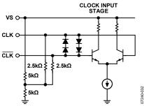
Figure 33. CLK Equivalent Input Circuit
