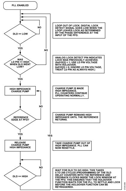
Figure 34. Flowchart of Automatic/Internal Holdover Mode
