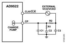
Figure 29. Example of External Loop Filter for PLL
