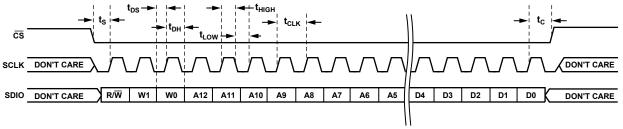
Figure 53. Serial Control Port Read—MSB First, 16-Bit Instruction, Timing Measurements
