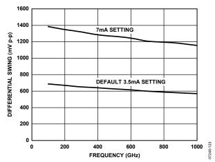
Figure 17. LVDS Differential Voltage Swing vs. Frequency, Output Terminated 100 Ω Across Differential Pair
