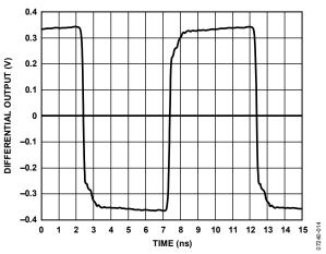
Figure 13. LVDS Output (Differential) at 100 MHz, Output Terminated 100  $\Omega$  Across Differential Pair
