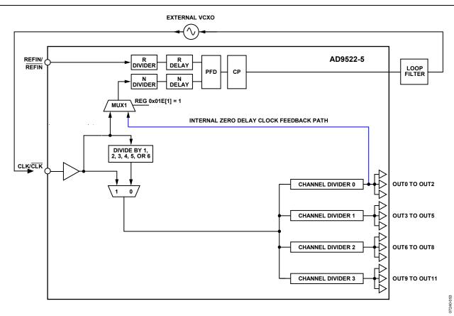
Figure 36. Zero Delay Function
