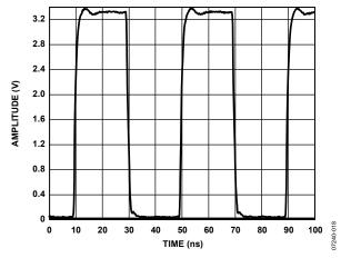
Figure 15. CMOS Output with 10 pF Load at 25 MHz
