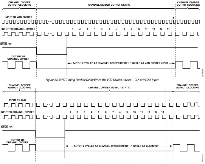
Figure 40. SYNC Timing Pipeline Delay When the VCO Divider Is Not Used
