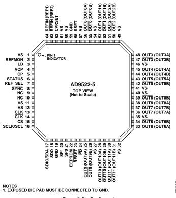
Figure 5. Pin Configuration
