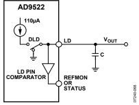
Figure 32. Current Source Digital Lock Detect
