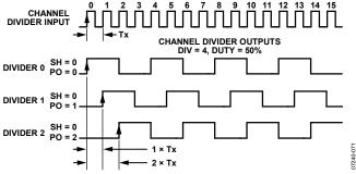
Figure 38. Effect of Coarse Phase Offset (or Delay)
