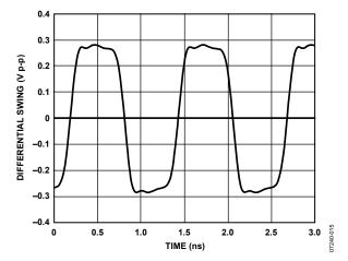
Figure 14. LVDS Differential Voltage Swing at 800 MHz, Output Terminated 100 Ω Across Differential Pair
