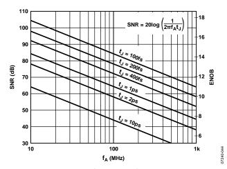
Figure 57. SNR and ENOB vs. Analog Input Frequency
