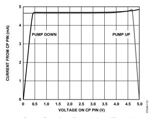
Figure 9. Charge Pump Characteristics at VCP = 5.0 V
