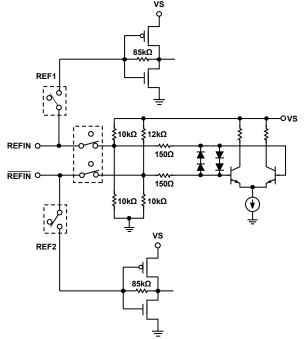
Figure 30. REFIN Equivalent Circuit for Non-XTAL Mode
