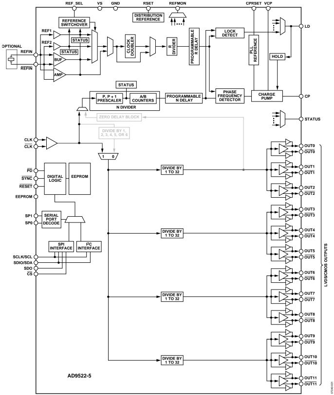
Figure 26. Clock Distribution or External VCO < 1600 MHz (Mode 1)
