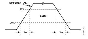
Figure 3. LVDS Timing, Differential
