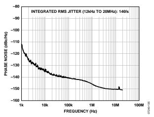
Figure 24. Phase Noise (Absolute), External VCXO (Toyocom TCO-2112) at 245.76 MHz; PFD = 15.36 MHz; LBW = 250 Hz; LVDS Output = 245.76 MHz
