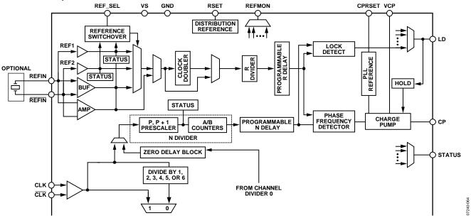
Figure 28. PLL Functional Block Diagram
