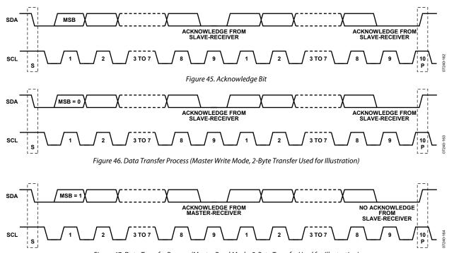
Figure 47. Data Transfer Process (Master Read Mode, 2-Byte Transfer Used for Illustration)
