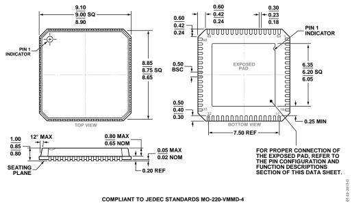
Figure 61. 64-Lead Lead Frame Chip Scale Package [LFCSP\_VQ] 9 mm × 9 mm Body, Very Thin Quad CP-64-4 Dimensions shown in millimeters
