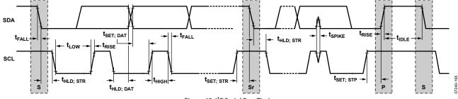
Figure 48. I<sup>2</sup>C Serial Port Timing
