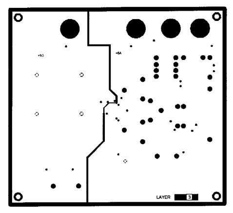
Figure 30. Power Plane PCB Layout (Layer 3)
