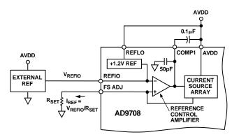
Figure 14. External Reference Configuration
