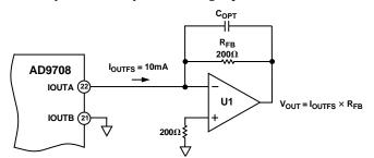
Figure 17. Unipolar Buffered Voltage Output
