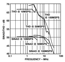
Figure 6. SINAD/THD vs. four (AVDD and DVDD = 3.0 V
