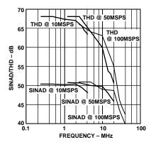
Figure 3. SINAD/THD vs. f<sub>OUT</sub> (AVDD and DVDD = 5.0 V
