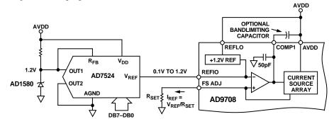
Figure 15. Single-Supply Gain Control Circuit
