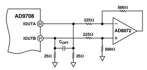
Figure 24. DC Differential Coupling Using an Op Amp
