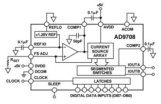
Differential current outputs are provided to support singleended or differential applications. The current outputs may be directly tied to an output resistor to provide two complementary, single-ended voltage outputs. The output voltage compliance range is 1.25 V.
