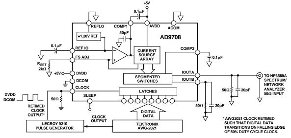
Figure 2. Basic AC Characterization Test Setup
