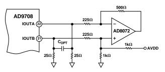
Figure 25. Single-Supply DC Differential Coupled Circuit
