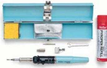
Butane gas operated, self igniting soldering iron with solder and hot blow functions. The tool has a rapid heat up time and one filling lasts up to 3 hours. It is temperature variable between 350°C to 500°C when used as a soldering iron and up to 650°C when used as a hot air blower.
