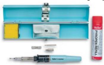
Manually ignited butane gas operated, soldering iron with solder, hot blow and blow torch functions. The tool has a rapid heat up time and duration of operation from one filling of approx. 3 hours. It is temperature variable between 350°C to 500°C when used as a soldering iron and up to 650°C when used as a hot air blower and 1300°C when used as a blow torch.
