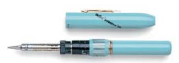
Manual ignited lightweight Butane gas operated soldering iron with solder, hot blow and blow torch functions. Supplied with aluminium protective cap with pocket clip and safety feature to prevent the cap being fitted when the iron is on. Temperature variable between 400°C to 500°C when used as a soldering iron, up to 650°C when used as a hot air blower and 1300°C when used as a blow torch.
