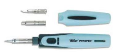
An ergonomic Butane gas operated soldering iron with solder, hot blow and blow torch functions. Offers maximum flexibility for use in many applications. It is temperature variable within the range of 500°C to 1300°C dependant upon the function used. Refilling takes only a few seconds and it operates approx. 1 hour with one filling. An integral sight glass shows the level of the gas in the tank. Ignition of the gas requires an external source and the long life tips deliver rapid heat up.
