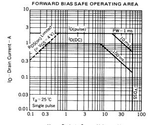
$V_{\mbox{DS}}-\mbox{Drain}$  to Source Voltage-V
