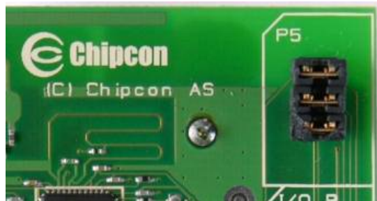
Figure 5: P5 default jumper settings
