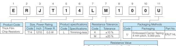
The first two digits are significant figures of resistance and the third one denotes number of zeros following. Example:  $222\rightarrow2.2~\text{k}\Omega$
