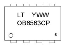
Y:Year Code(0-9) WW:Week Code(01-52) C:SOP8 Package P:Pb-free Package S:Internal Code(Optional)
