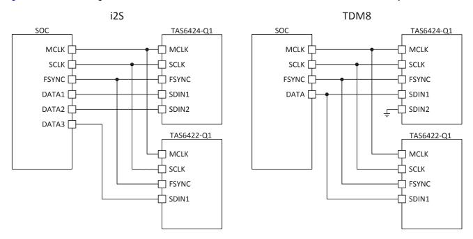
Figure 35. Digital-Audio Data Connection
