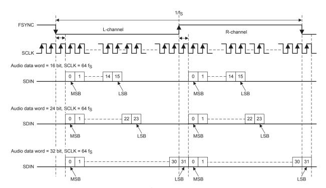
Figure 38. I<sup>2</sup>S Audio Data Format
