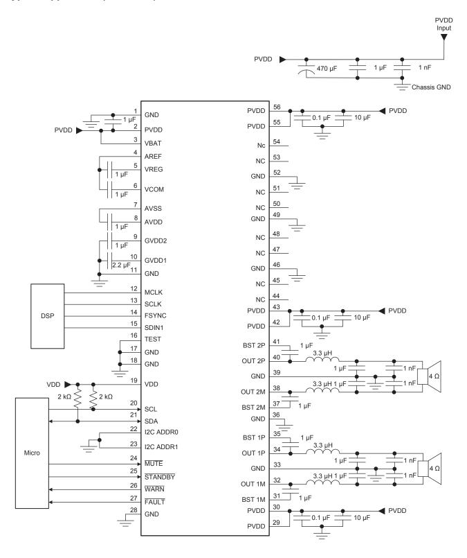
Figure 77. Typical 2-Channel BTL Application Schematic
