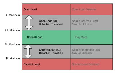
Figure 40. DC Load Diagnostic Reporting Thresholds
