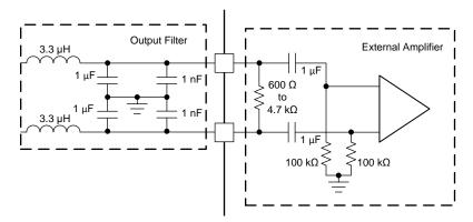
Figure 76. External Amplifier Input Configuration for Line Driver
