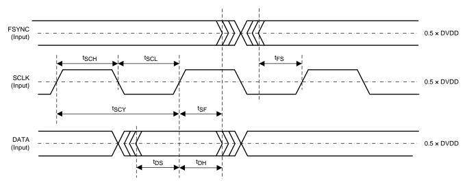
Figure 36. Serial Audio Timing
