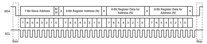
Figure 41. Typical I<sup>2</sup>C Sequence
