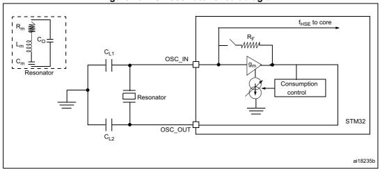
Figure 15. HSE oscillator circuit diagram
