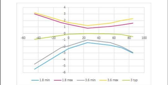
Figure 17. HSI16 minimum and maximum value versus temperature
