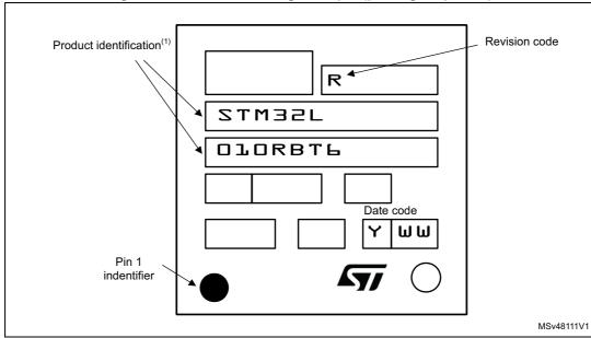
Figure 29. LQFP64 marking example (package top view)
