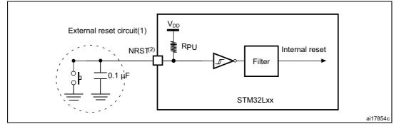
Figure 21. Recommended NRST pin protection
