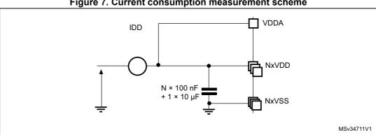
Figure 7. Current consumption measurement scheme
