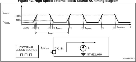
Figure 13. High-speed external clock source AC timing diagram
