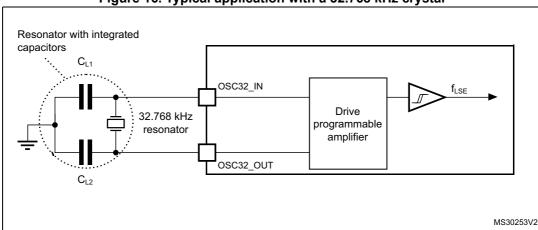
Figure 16. Typical application with a 32.768 kHz crystal
