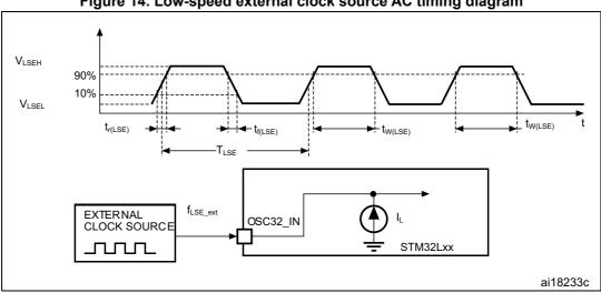
Figure 14. Low-speed external clock source AC timing diagram
