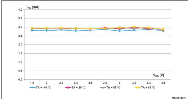
Figure 9.  $I_{DD}$  vs  $V_{DD}$ , Run mode, code running from Flash memory, Range 2, HSE bypass, 1 ws
