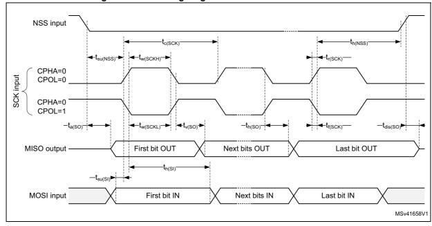
Figure 24. SPI timing diagram - slave mode and CPHA = 0
