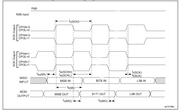
Figure 26. SPI timing diagram - master mode<sup>(1)</sup>
