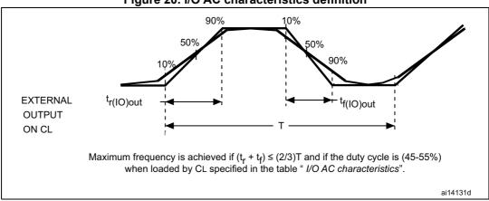
Figure 20. I/O AC characteristics definition
