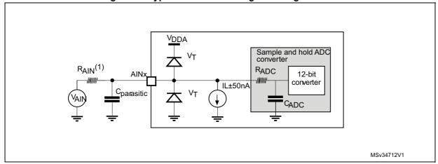
Figure 23. Typical connection diagram using the ADC
