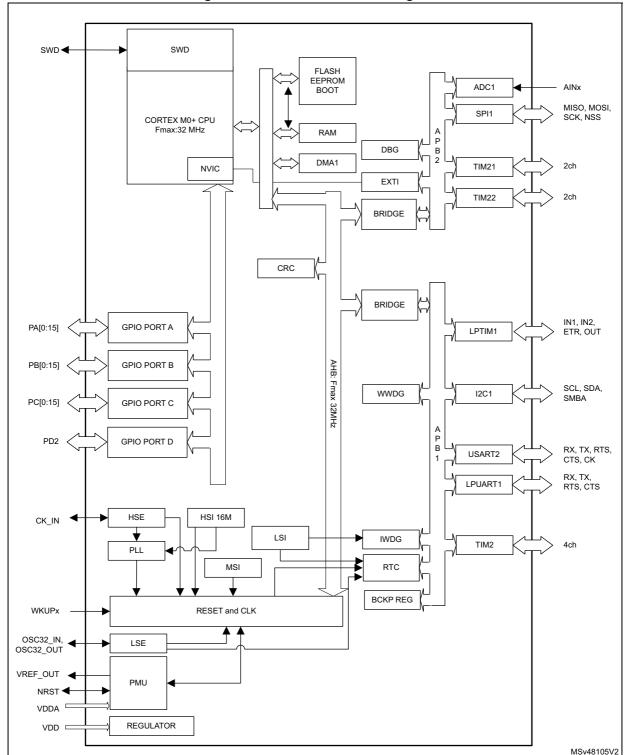
Figure 1. STM32L010RB block diagram
