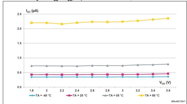
Figure 12.  $I_{DD}$  vs  $V_{DD}$ , Stop mode with RTC disabled, all clocks off
