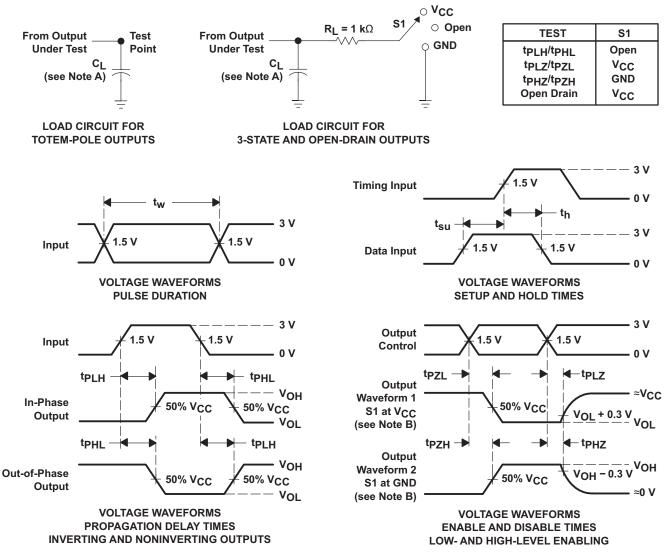
CL includes probe and jig capacitance.
