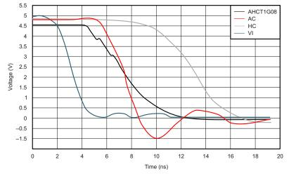
$V_{CC} = 5 V$  Load = 50  $\Omega$  / 50 pF
