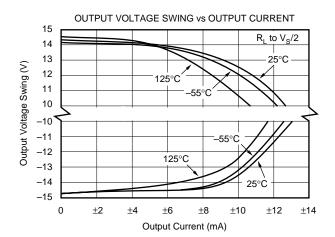
At  $T_A$  = 25°C,  $V_S$  = +15V, and  $R_L$  = 20k $\Omega$  connected to Ground, unless otherwise noted.
