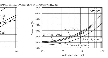
At  $T_A$  = 25°C,  $V_S$  = +15V, and  $R_L$  = 20k $\Omega$  connected to Ground, unless otherwise noted.
