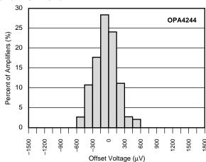
At  $T_A$  = 25°C,  $V_S$  = +15V, and  $R_L$  = 20k $\Omega$  connected to Ground, unless otherwise noted.
