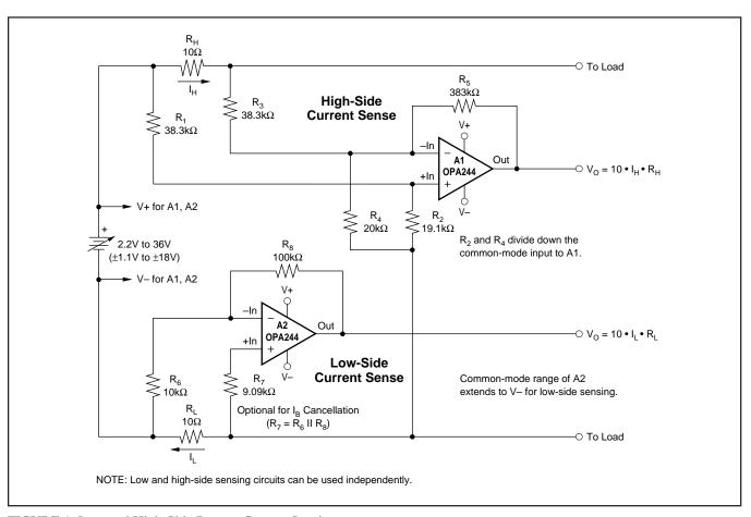
FIGURE 1. Low and High-Side Battery Current Sensing.
