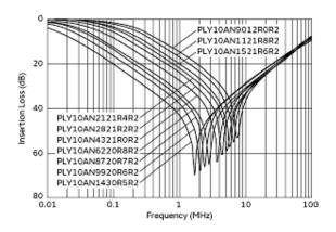
Differential Mode Insertion Loss-Frequency Characteristics
