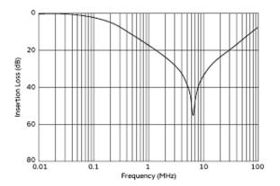
Common Mode Insertion Loss (Typ.)
