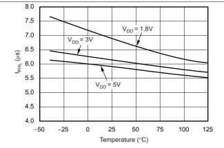
Figure 11. Propagation Delay ( $t_{PLH}$ ) vs Temperature
