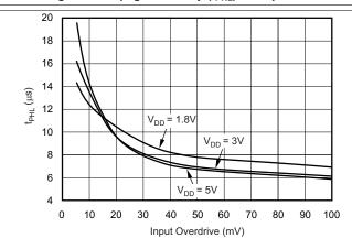
Figure 9. Propagation Delay (t<sub>PLH</sub>) vs Input Overdrive
