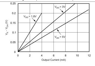
Figure 5. Output Low vs Output Current
