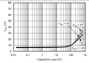
Figure 7. Propagation Delay (t<sub>PLH</sub>) vs Capacitive Load
