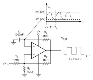
Figure 20. TLV349x Configured as a Relaxation Oscillator
