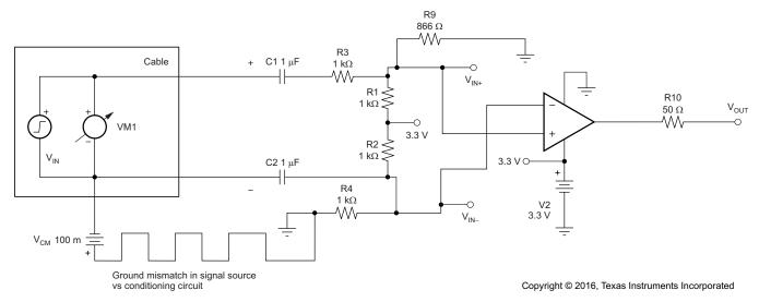
Figure 18. TLV3491 Configured as an AC-Coupled Comparator (Schematic)
