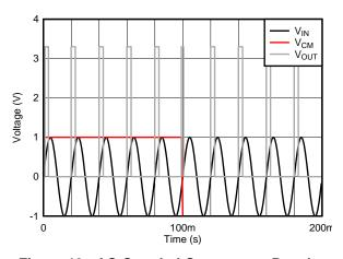
Figure 19. AC-Coupled Comparator Results
