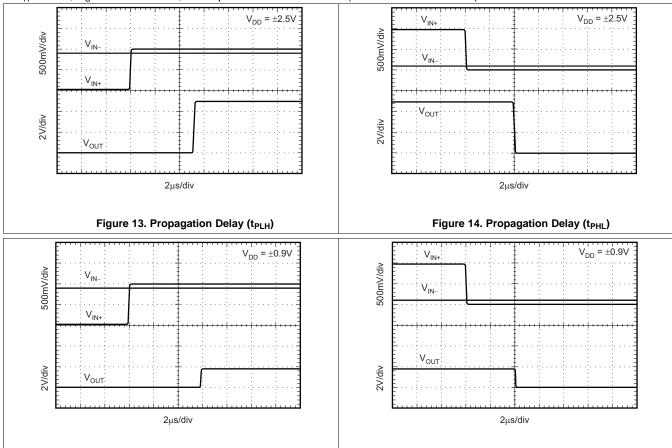
Figure 15. Propagation Delay (t<sub>PLH</sub>)
