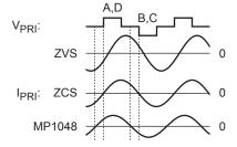
Figure 2—V<sub>PRI</sub> vs. I<sub>PRI</sub>
