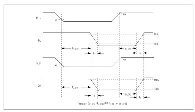
Figure 1. Timing Characteristics of Logic Inputs (MAX15018A/MAX15019A)
