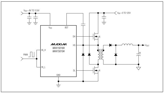
Figure 3. Two-Switch Forward Application
