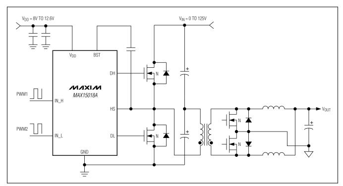
Figure 2. Half-Bridge Converter Application with Secondary-Side Synchronous Rectification
