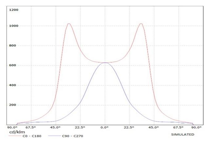
Luminaire: Ledil CA10925 STRADA-B\_(XM-L) Lamps: 1 x Cree\_XM-L\_(XMLAWT-00-0000-0000T6051) \_102.237lm@250mA\_CCT=8850K\_P=0.7W\_I=0.25A
