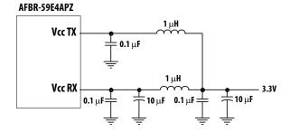
Note: Inductors should have less than  $1\Omega$  series resistor per MSA.
