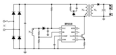
Figure 1. Typical application circuit for BP3318
