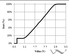
Output LED Current vs. DIM pin voltage
