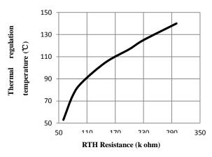
Thermal Regulation Temperature vs. RTH pin
