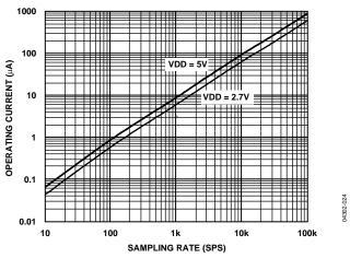
Figure 24. Operating Current vs. Sampling Rate
