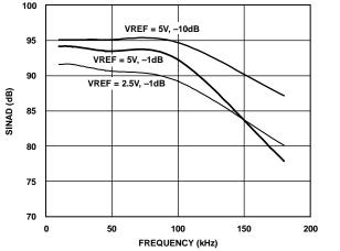
Figure 14. SINAD vs. Frequency
