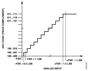
Figure 21. ADC Ideal Transfer Function
