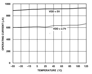
Figure 17. Operating Current vs. Temperature
