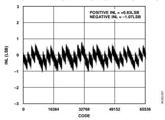
Figure 7. Integral Nonlinearity vs. Code
