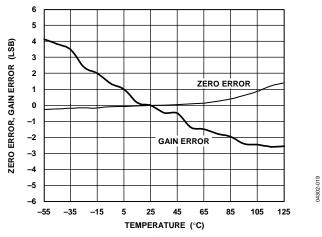
Figure 19. Zero Error and Gain Error vs. Temperature
