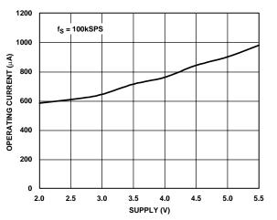
Figure 16. Operating Current vs. Supply
