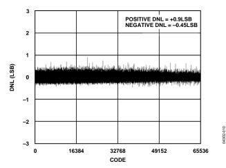
Figure 10. Differential Nonlinearity vs. Code
