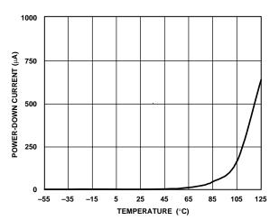
Figure 18. Power-Down Current vs. Temperature
