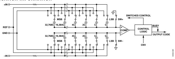
Figure 20. ADC Simplified Schematic
