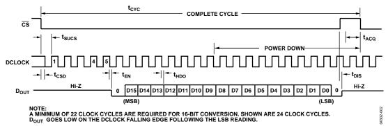
Figure 2. Serial Interface Timing
