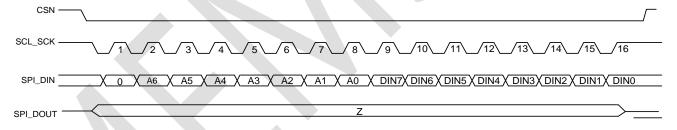
Figure 14. SPI Register Write Cycle - Single
