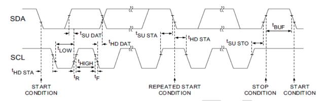
Figure 10. I2C Interface Timing
