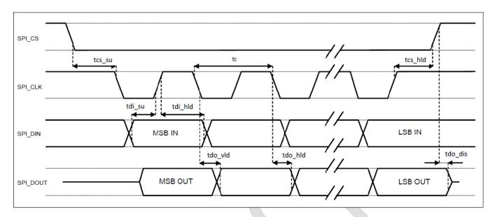
Figure 18. SPI Interface Timing
