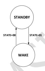
Figure 11. Operational State Flow
