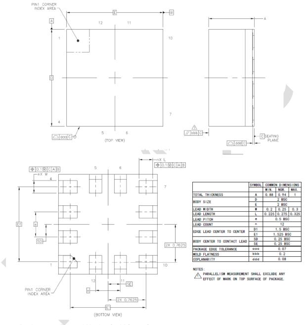
Figure 2. Package Outline and Mechanical Dimensions
