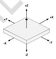
Figure 4. Package Axis Reference
