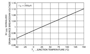
Figure 7. Breakdown Voltage Variation with Temperature.
