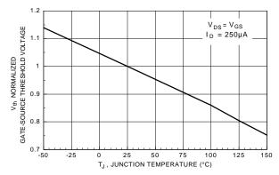
Figure 6. Gate Threshold Variation with Temperature.
