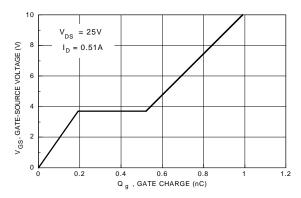
Figure 10. Gate Charge Characteristics.
