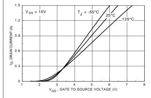
Figure 5. Transfer Characteristics.
