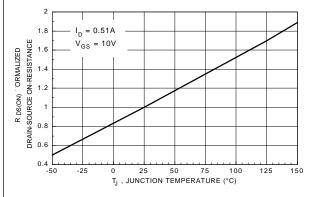
Figure 3. On-Resistance Variation with Temperature.
