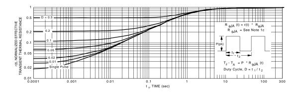
Figure 15. Transient Thermal Response Curve.
