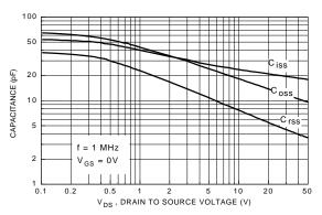
Figure 9. Capacitance Characteristics.
