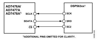
Figure 30. Interfacing to the DSP563xx
