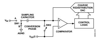
Figure 16. ADC Conversion Phase
