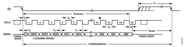
Figure 24. AD7476A Serial Interface Timing Diagram
