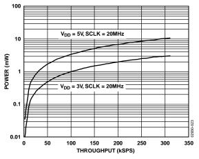
Figure 23. Power vs. Throughput
