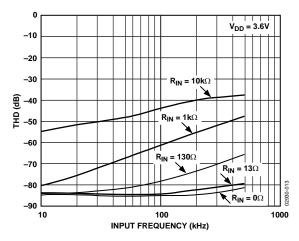
Figure 13. THD vs. Analog Input Frequency for Various Source Impedances
