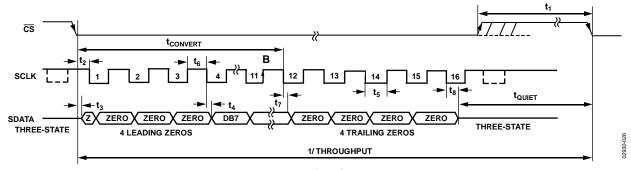
Figure 26. AD7478A Serial Interface Timing Diagram
