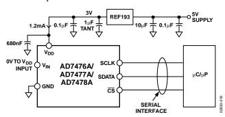
Figure 18. REF193 as Power Supply to AD7476A/ AD7477A/AD7478A
