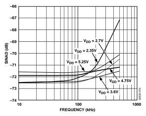
Figure 10. AD7476A SINAD vs. Input Frequency at 1 MSPS
