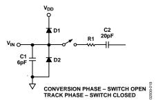
Figure 19. Equivalent Analog Input Circuit
