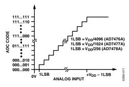
Figure 17. AD7476A/AD7477A/AD7478A Transfer Characteristic
