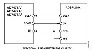
Figure 29. Interfacing to the ADSP-218x
