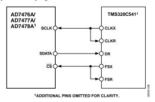
Figure 28. Interfacing to the TMS320C541
