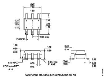
Figure 33. 6-Lead Thin Shrink Small Outline Transistor Package [SC70] (KS-6) Dimensions shown in millimeters
