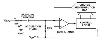
Figure 15. ADC Acquisition Phase
