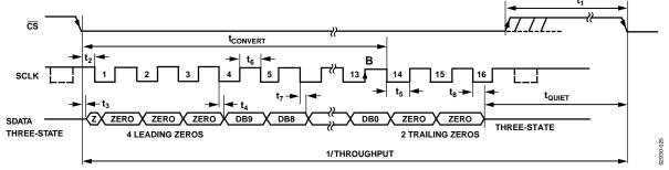
Figure 25. AD7477A Serial Interface Timing Diagram
