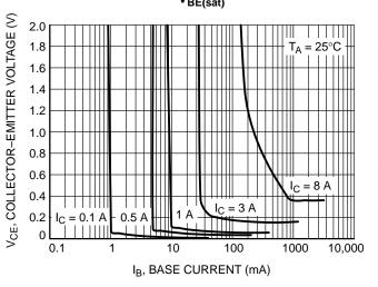
Figure 12. MJD44H11 Collector Saturation Region
