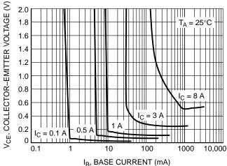
Figure 13. MJD45H11 Collector Saturation Region
