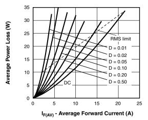
Fig. 6 - Forward Power Loss Characteristics
