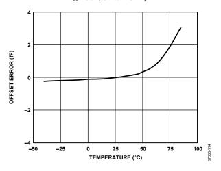
Figure 14. Capacitance Input Offset Error vs. Temperature,  $V_{DD} = 3.3 V$ , CIN and EXC Pins Open Circuit
