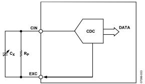
Figure 44. Parasitic Parallel Resistance
