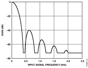
Figure 18. Capacitance to Digital Converter Frequency Response
