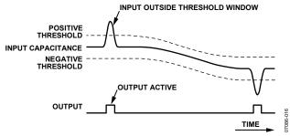
Figure 26. Out-Window (Adaptive) Threshold Mode
