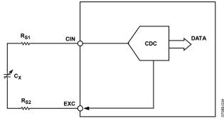
Figure 45. Parasitic Serial Resistance
