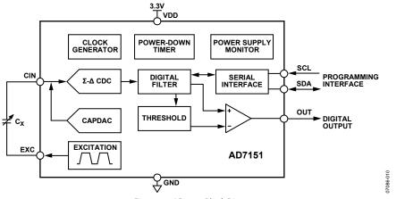
Figure 20. AD7151 Block Diagram
