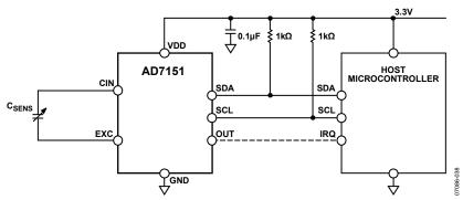
Figure 50. AD7151 Interfaced to a Host Microcontroller
