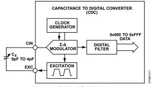
Figure 21. CDC Simplified Block Diagram
