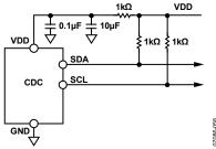
Figure 48. AD7151 V<sub>DD</sub> Decoupling and Filtering
