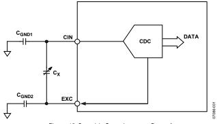
Figure 42. Parasitic Capacitance to Ground
