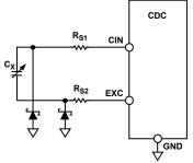
Figure 46. AD7151 CIN Overvoltage Protection
