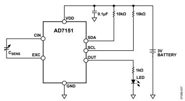
Figure 49. AD7151 Standalone Operation Application Diagram
