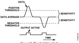
Figure 35. Threshold Sensitivity
