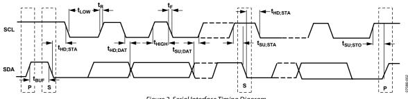
Figure 2. Serial Interface Timing Diagram
