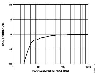
Figure 13. Capacitance Input Gain Error vs. Parallel Resistance,  $V_{DD} = 3.3 V$ , CIN to EXC = 2 pF
