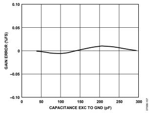
Figure 7. Capacitance Input Gain Error vs. Capacitance EXC to GND,  $V_{\text{DD}}$  = 3.3 V, CIN to EXC = 2 pF
