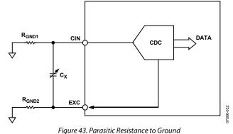
The AD7151 CDC result is affected by a leakage current from  $C_x$  to ground; therefore,  $C_x$  should be isolated from the ground. The equivalent resistance between  $C_x$  and ground should be maximized (see Figure 43).
