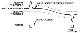
Figure 25. In-Window (Adaptive) Threshold Mode
