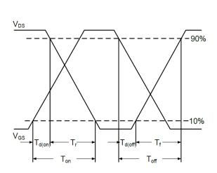
Figure 10. Switching Time Waveform
