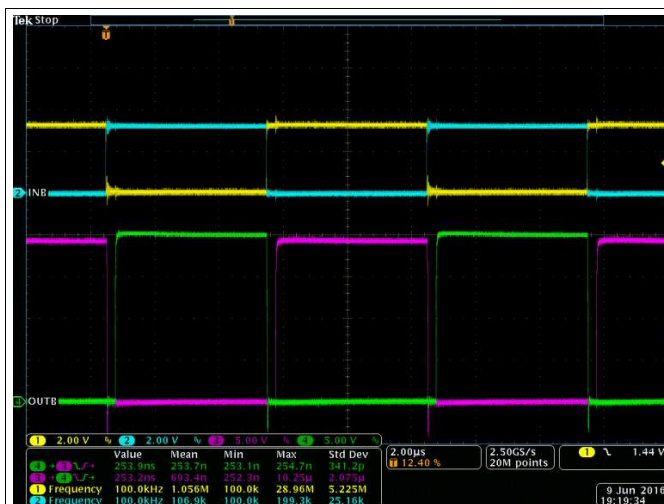
Figure 42. Bench Test Waveform for INA/B and OUTA/B
