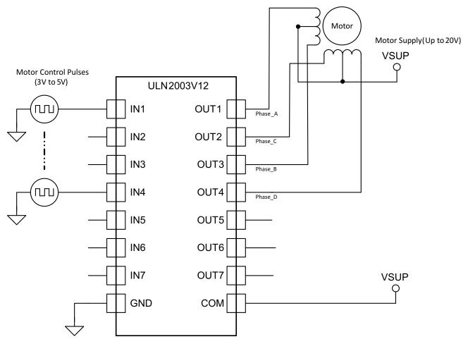
Figure 7. ULN2003V12 as a Stepper Motor Driver
