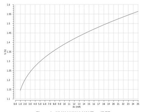
Figure 6. ULN2003V12 VOUT vs IREF
