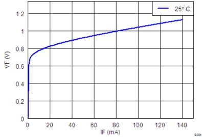
Figure 11. Freewheeling Diode VF versus IF
