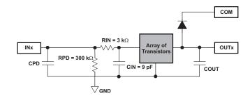
Figure 2. Channel Block Diagram
