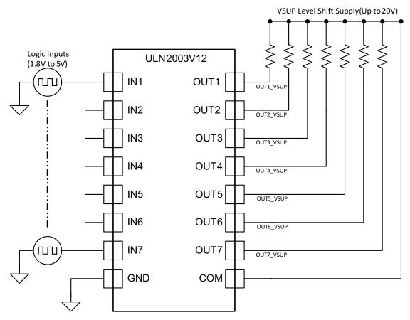
Figure 3. ULN2003V12 as Inverting Logic Level Shifter
