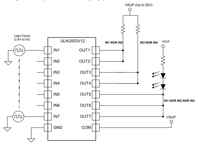
Figure 8. ULN2003V12 as a NOR driver
