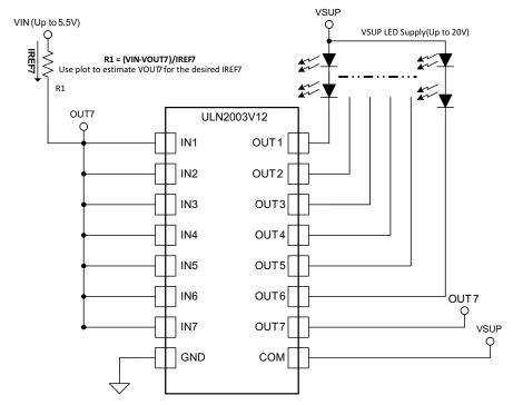
Figure 5. ULN2003V12 as a Constant Current Driver
