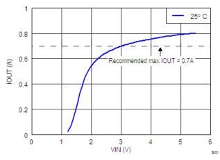
Figure 9. Load Current 1-Channel; VOL=0.6V
