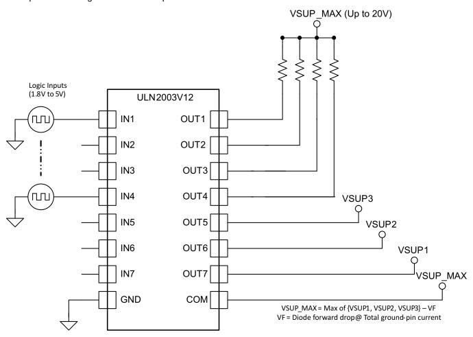
Figure 4. ULN2003V12 as Max Supply Selector
