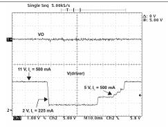
Figure 11. Input Voltage Excursions (Similar to Low-Crank Conditions)
