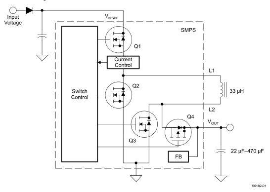
Figure 18. Buck/Boost Switch Mode Configuration
