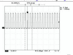
Figure 13. Nominal Switching Frequency of Q1 Switch (446 kHz) With Modulation Function Disabled,  $I_L=200\ mA$
