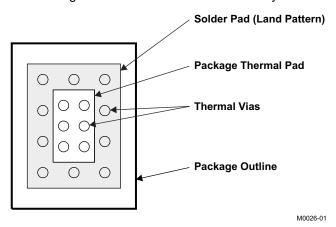
Figure 23. Package and PCB Land Configuration for a Multilayer PCB
