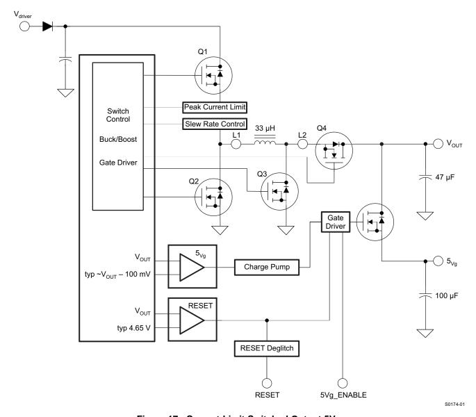
Figure 17. Current-Limit Switched Output 5Vg
