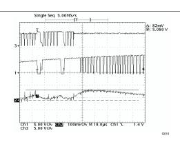
Figure 14. Switched-Mode Regulator Transition from Boost Mode to Buck Mode,  $I_L$  = 400 mA
