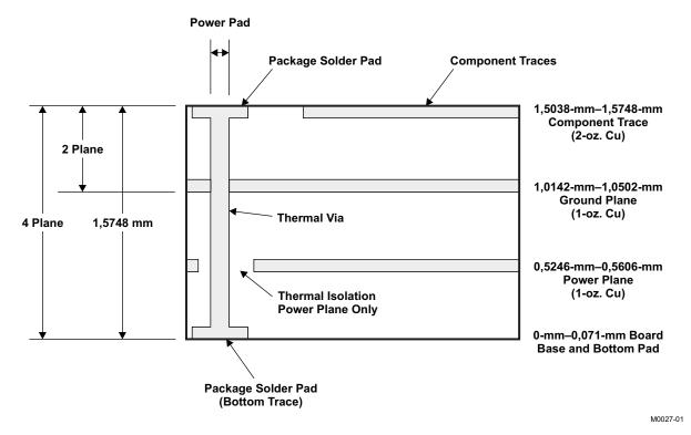
Figure 24. Multilayer Board (Side View)
