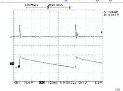
Figure 7. Low-Power-Mode Operation,  $I_L$  = 15 mA,  $C_O$  = 47  $\mu F$
