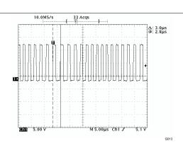
Figure 8. Minimum Switching Frequency (333 kHz) with Modulation Enabled,  $R_{mod} = 12 \text{ k}\Omega$ ,  $I_L = 200 \text{ mA}$
