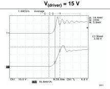
Figure 5. Input Current with Slope Control, SCR1 = 1, SCR0 = 0, Input-Current Slew Rate = 9.4 A/ $\mu$ s, I<sub>L</sub> = 500 mA, V<sub>(driver)</sub> = 15 V
