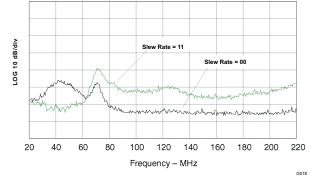
These values represent conducted EMI results of a test board for display purposes only. Actual results may vary greatly depending on board layout and external components and must be verified in actual application.
