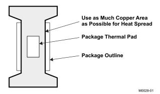
Figure 25. Land Configuration for Single-Layer PCB
