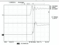
Figure 6. Input Current With Slope Control, SCR0 = 1, SCR1 = 1, Input-Current Slew Rate = 18.8 A/ $\mu$ s, I<sub>L</sub> = 500 mA,  $V_{(driver)}$  = 15 V
