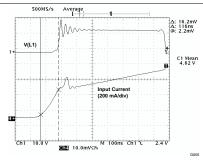
Figure 3. Input Current with Slope Control, SCR0 = 0, SCR1 = 0, Input-Current Slew Rate = 2.8 A/ $\mu$ s, I<sub>L</sub> = 500 mA,
