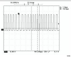
Figure 9. Maximum Switching Frequency (555 kHz) With Modulation Enabled,  $R_{mod}$  = 12 k $\Omega$ ,  $I_L$  = 200 mA
