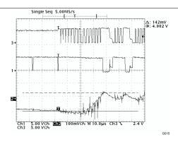
Figure 12. Switched-Mode Regulator Transition from Buck Mode to Boost Mode,  $I_L$  = 400 mA
